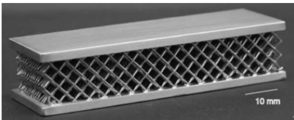
Fig. 9. An example of a diamond orientation, 304 stainless steel textile sandwich panel. The core relative density was 12.6%.
