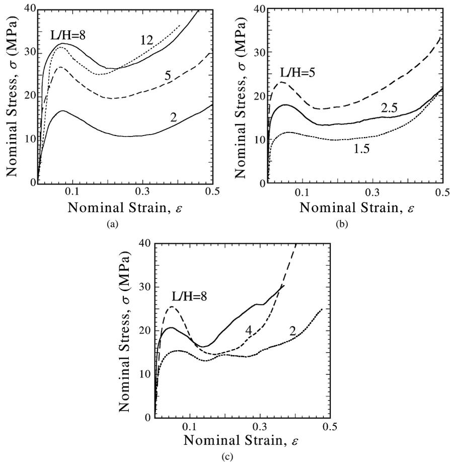
Fig. 5. Nominal compressive stress versus strain response of the woven core sandwich plates (a)  $\bar{\rho} = 0.23$  ( $H/d = 5$ ), (b)  $\bar{\rho} = 0.20$  ( $H/d = 8$ ) and (c)  $\bar{\rho} = 0.18$  ( $H/d = 5$ ). In all cases, the width to height ratio is  $W/H = 1$ .
