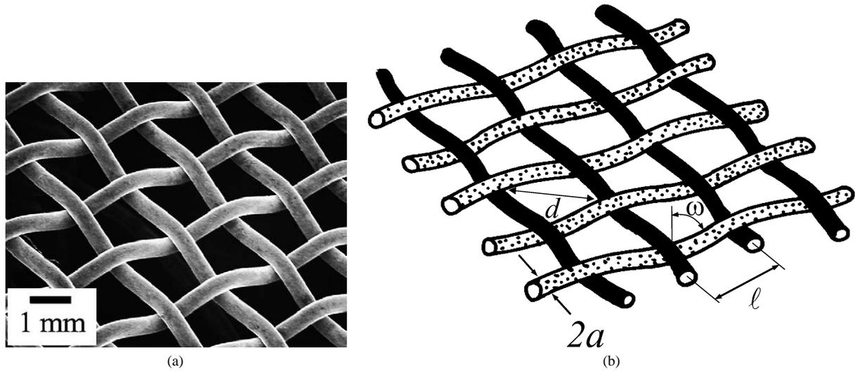
Fig. 1. (a) Photograph of 316 stainless steel wire mesh used to manufacture the woven cores; (b) Sketch of the wire mesh of wire radius  $a$ , cell diagonal length  $d$ , cell size  $l$  and weave angle  $\omega$ .
