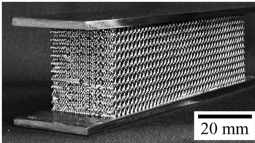
Fig. 4. Photograph of a sandwich plate with a woven core of relative density  $\bar{\rho} = 0.23$  manufactured from 316 stainless steel wire mesh.
