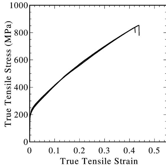
Fig. 9. Measured tensile stress versus strain response of the as-brazed 316 stainless steel.
