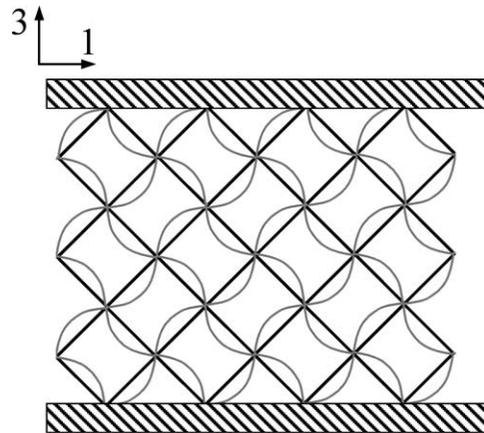
Fig. 3. Sketch of the assumed plastic buckling mode (gray lines) of the wire mesh.
