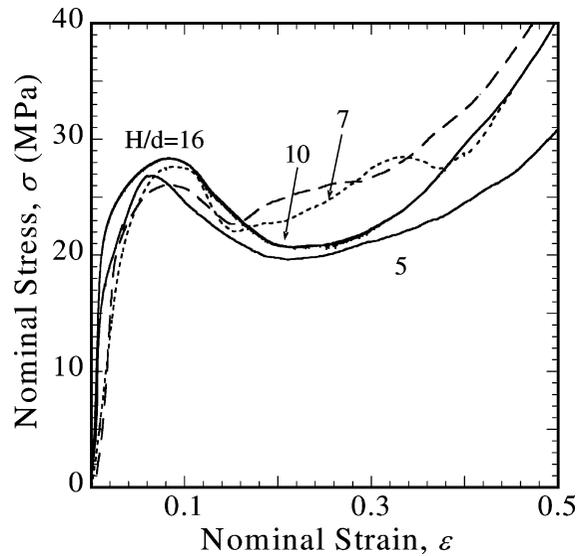
Fig. 6. The effect of specimen height to cell size ratio  $H/d$ , on the compressive stress versus strain response. The relative density is  $\bar{\rho} = 0.23$ , the aspect ratio is  $L/H = 4$ , and the width to height ratio is  $W/H = 1$ .
