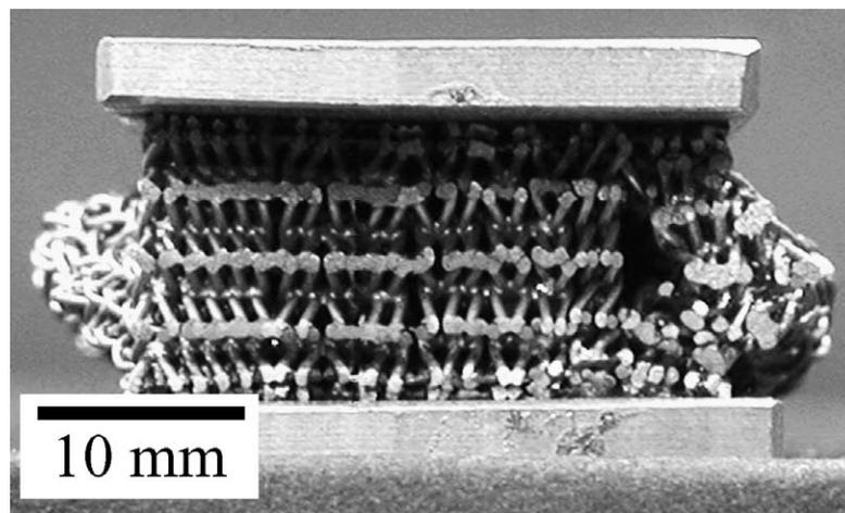
Fig. 7. A side view of a woven core specimen compressed to a strain  $\varepsilon \approx 40\%$  ( $\bar{\rho} = 0.23$ ,  $L/H = 4$ ,  $H/d = 7$  and  $W/H = 1$ ). The photograph indicates that two to four layers at the front and back faces of the specimen delaminate.
