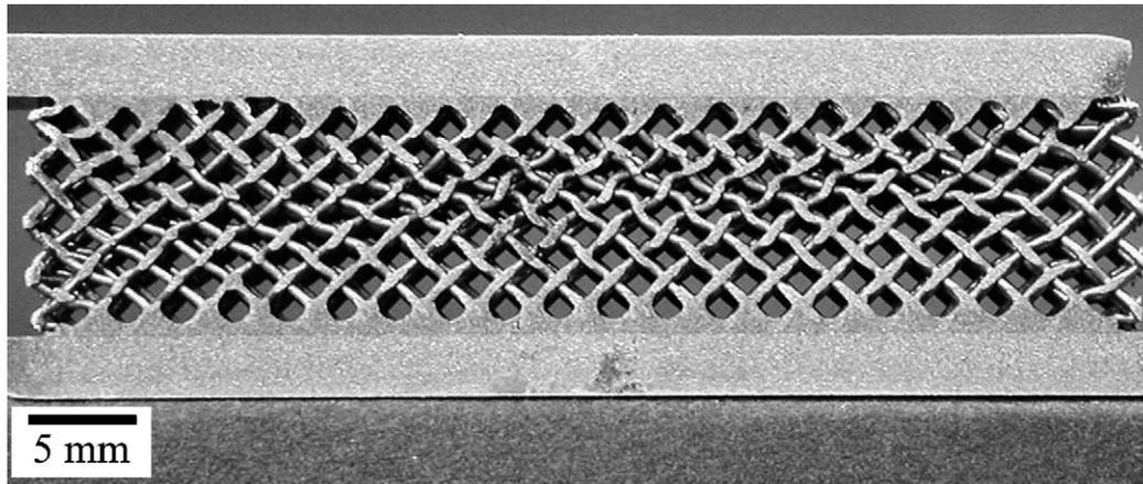
Fig. 11. Photograph of a woven core specimen compressed to just beyond the peak strength,  $\varepsilon \approx 11\%$ , and sectioned along its mid-plane. The photograph shows a buckling mode similar to that sketched in Fig. 3.  $\bar{\rho} = 0.23$ ,  $L/H = 4$ ,  $H/d = 5$  and  $W/H = 1$ .
