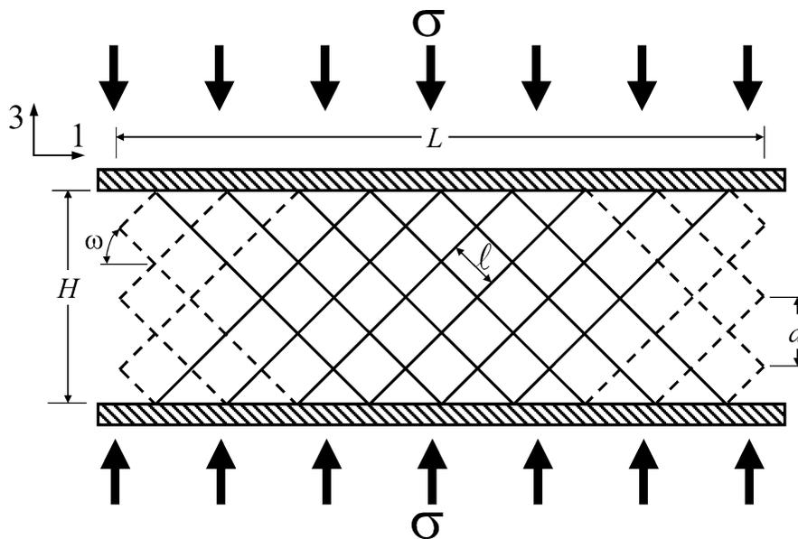
Fig. 2. Sketch of a woven core sandwich plate under out-of-plane compression. The solid lines are mesh wires that are bonded to both face sheets and carry load while the dashed lines are mesh wires that are bonded to one face sheet only and are assumed to carry no load in the lower bound analysis.
