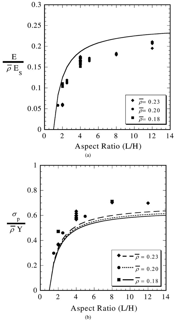
Fig. 10. Comparison of the measured and predicted (a) Young's modulus  $E$  and (b) peak collapse strength  $\sigma_p$  as a function of the aspect ratio of the sandwich core  $L/H$ .
