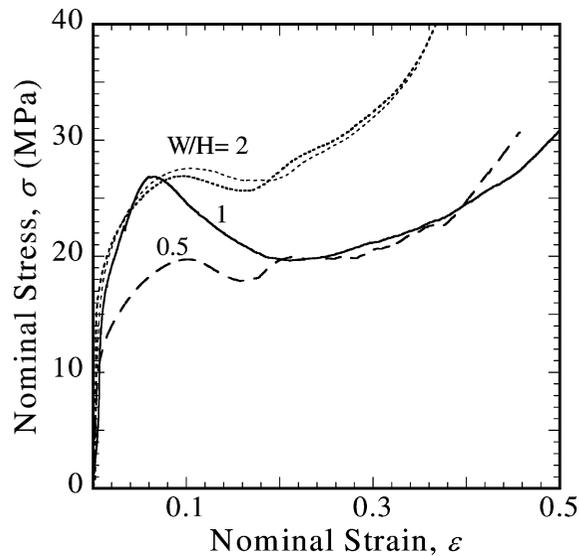
Fig. 8. The effect of specimen width to height ratio  $W/H$  upon the compressive stress versus strain response of woven core sandwich plates of relative density  $\bar{\rho} = 0.23$ , aspect ratio  $L/H = 4$  and height to cell size ratio  $H/d = 5$ .
