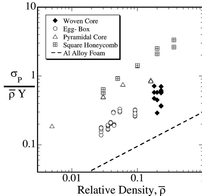
Fig. 12. Comparison of normalized core strength as a function of relative density for competing sandwich panel core topologies.
