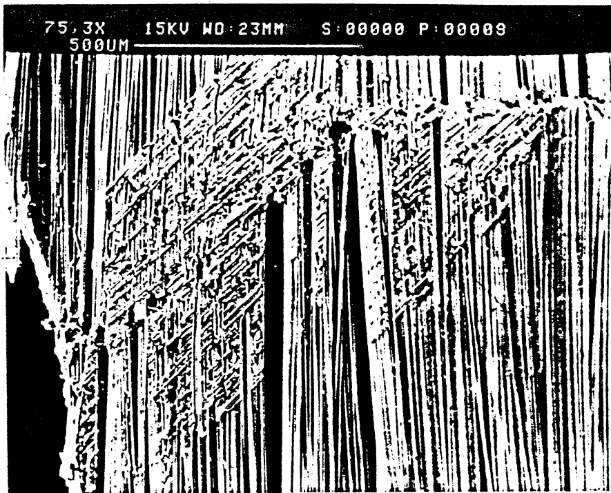
Fig.9 . a) Fibre microbuckling failure in a 0-deg ply. The line of fracture is initially at 45-deg to the loading axis. Applied strain 0.52%.
