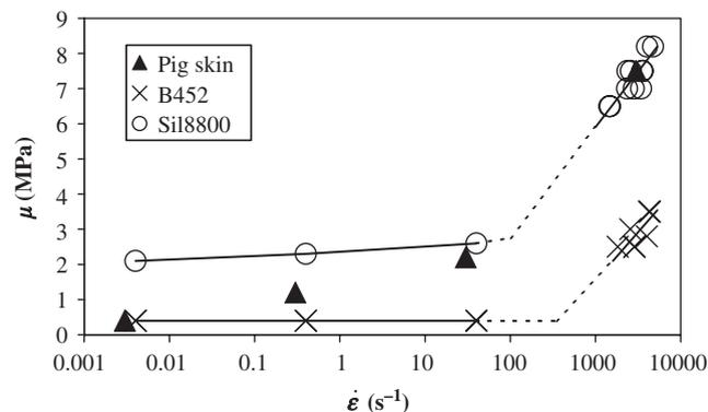
Fig. 8. Shear modulus versus strain rate response of pig skin and B452 and Sil8800 silicone rubber. There are insufficient data with which to construct a curve fitting line for the pig skin.
