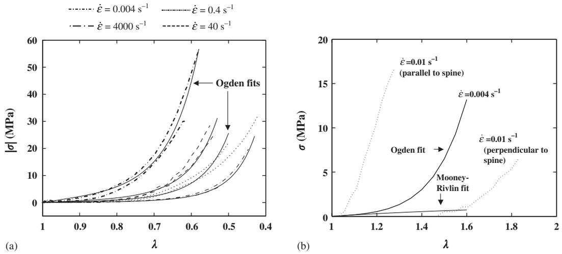
Fig. 5. The engineering stress versus stretch ratio response of pig skin to (a) uniaxial compression and (b) uniaxial tension.
