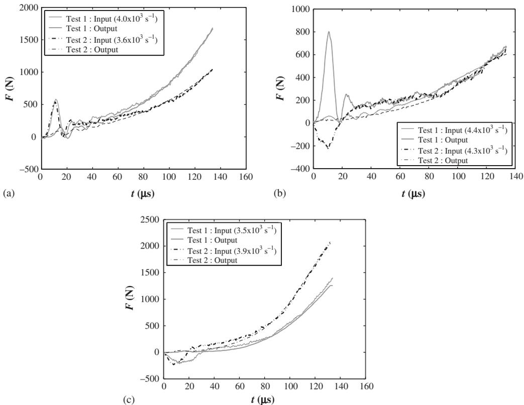
Fig. 9. Compressive force  $F$  versus time  $t$  response of (a) Sil8800, (b) B452 and (c) pig skin specimens tested at a strain rate of ca.  $\dot{\epsilon} = 4000 \text{ s}^{-1}$ .
