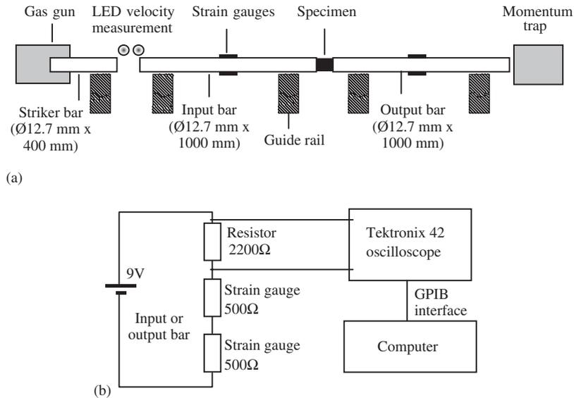
Fig. 3. (a) Sketch of a compressive split-Hopkinson pressure bar used for testing soft materials and (b) sketch of the circuit used for measuring the strain in the pressure bar by recording the change in the voltage across a resistor.
