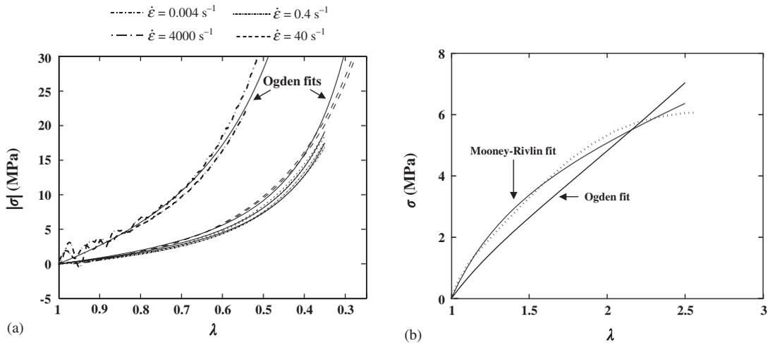
Fig. 7. The engineering stress versus stretch ratio response of Sil8800 silicone rubber to (a) uniaxial compression and (b) uniaxial tension.
