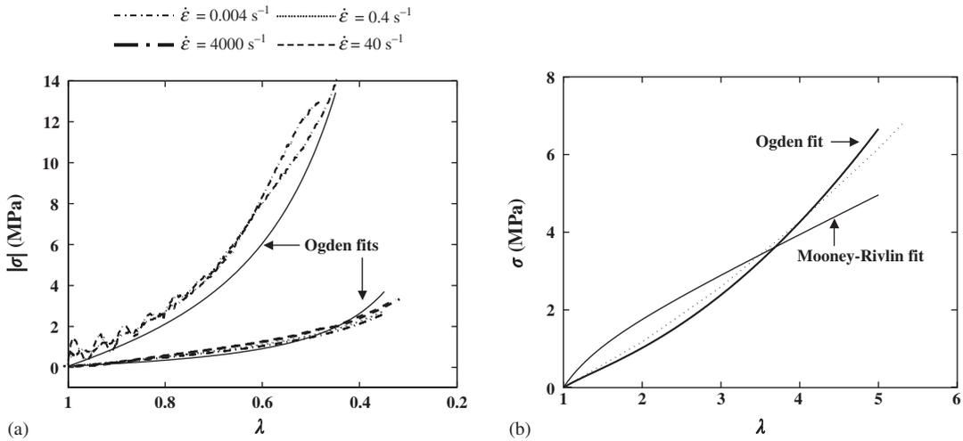
Fig. 6. The engineering stress versus stretch ratio response of B452 silicone rubber to (a) uniaxial compression and (b) uniaxial tension.
