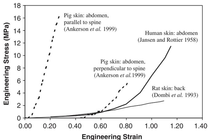
Fig. 1. Tensile uniaxial engineering stress versus engineering strain response for human, pig and rat skin.
