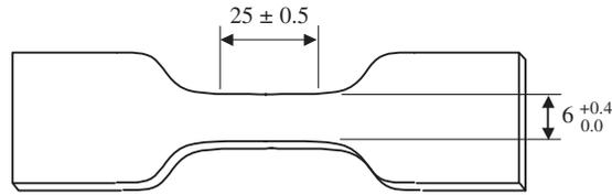
Fig. 4. Dog-bone specimen used for uniaxial tensile tests (dimensions in mm). Thickness = 2 mm.
