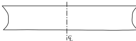
Fig. 2. Sketch of a silicone rubber specimen cut using an 8 mm diameter leather die punch. The punching operation results in a specimen with curved edges, reducing the effective diameter of the specimen.
