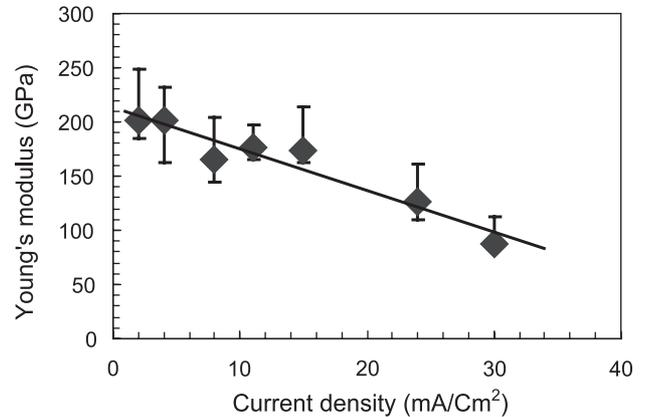
Fig. 4. Young's modulus as a function of plating current density plated at  $T=60$  °C.
