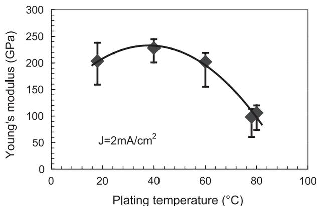
Fig. 3. Young's modulus of Ni thin film as a function of the plating temperature, with  $J=2$  mA/cm<sup>2</sup>.
