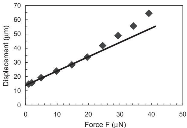
Fig. 2. The compliance of a representative cantilever Ni beam, electroplated at  $T=60$  °C and  $J=8$  mA/cm<sup>2</sup>.
