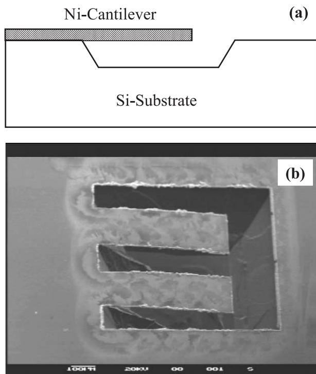
Fig. 1. The cross-sectional diagram (a) and SEM picture (b) of a Ni cantilever cut from an electroplated Ni film plate, and released by etching in KOH solution.
