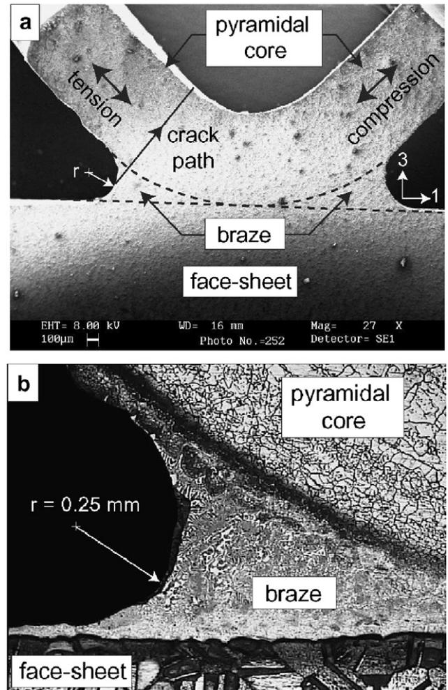
Fig. 6. (a) SEM photograph of a section of an undamaged joint showing the fatigue crack growth path starting at the toe of the braze joint of struts carrying tensile load. (b) Optical photograph of a polished braze joint showing the effect of diffusion bonding on the microstructure in the face-sheet and the pyramidal core. The radius arm of  $r = 0.25$  mm forms a suitable scale bar for the image.
