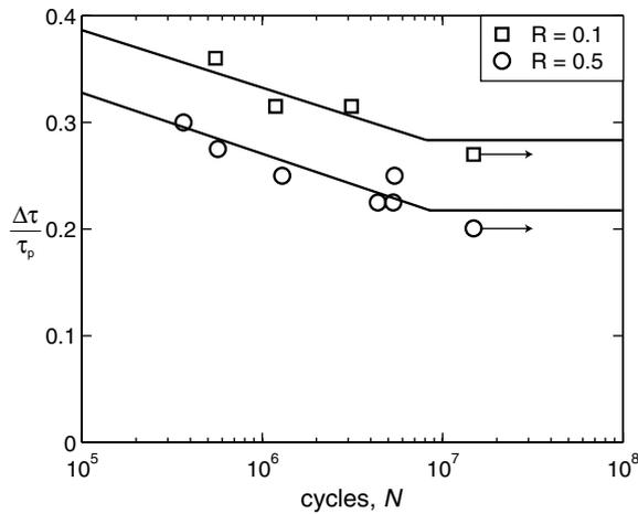
Fig. 7.  $S$ - $N$  curves of pyramidal core in longitudinal shear loading for loading ratio  $R = 0.1$  and  $0.5$ .
