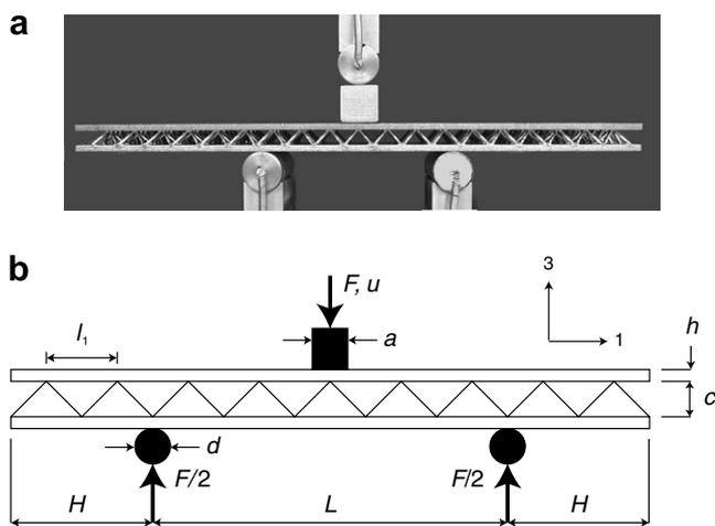
Fig. 10. (a) Photograph of a manufactured sandwich beam in three-point bending configuration with face-sheet thickness  $h = 2.95$  mm, span  $L = 90$  mm and core height  $c = 7.05$  mm (specimen  $S_1$ ). (b) Sketch of pyramidal core sandwich beam showing the parameters involve in a three-point bending test.
