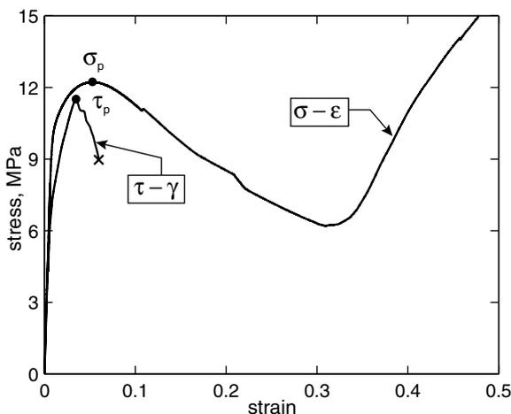
Fig. 3. The measured out-of-plane compressive response and longitudinal shear response of the  $\bar{\rho} = 0.066$  AL6XN pyramidal core.
