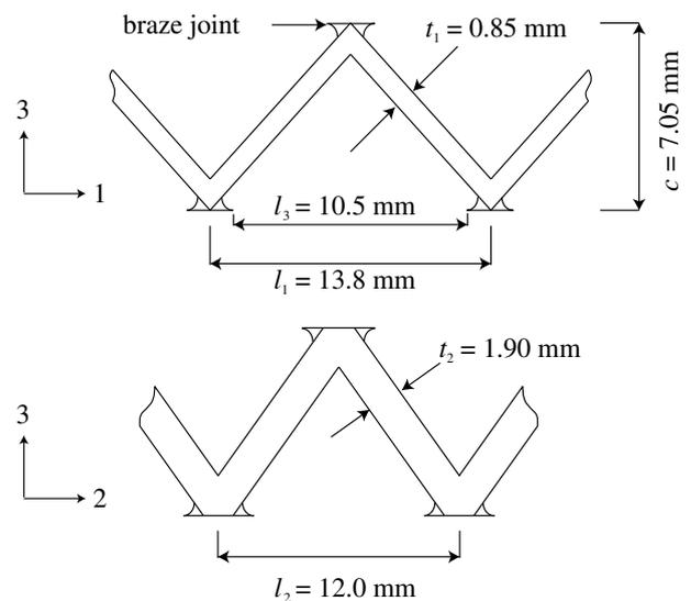
Fig. 2. Dimensions of the pyramidal core used in the present study.
