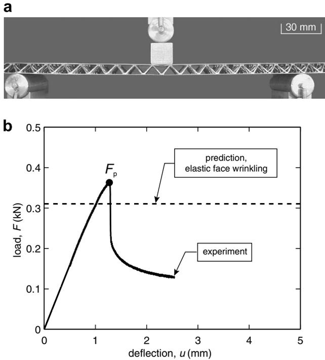
Fig. 12. (a) Photograph of a monotonically loaded deformed specimen with  $h = 0.3$  mm and  $L = 220$  mm. It collapses by elastic face wrinkling. (b) The  $F$  versus  $u$  response for this specimen along with the analytical prediction of the collapse strength.
