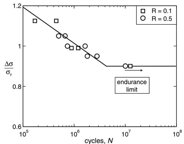
Fig. 9. The measured  $S$ - $N$  curves for brazed 304 stainless steel under tension-tension cyclic loading for the load ratio  $R = 0.1$  and  $0.5$ .
