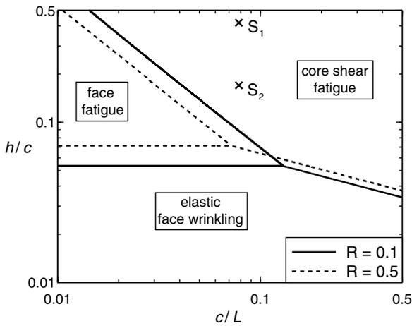
Fig. 15. The fatigue failure mechanisms map with  $h/c$  and  $c/L$  as axes for a sandwich beam with AL6XN pyramidal core of relative density  $\bar{\rho} = 0.066$ , using the measured material properties and beam geometries  $H/L = 1/4$  and  $a/L = 1/16$ . The specimens  $S_1$  and  $S_2$  denote the tested geometries in cyclic loading. Maps are shown for two different loading ratios:  $R = 0.1$  and  $R = 0.5$ .
