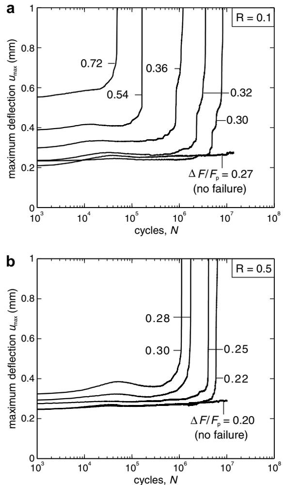
Fig. 16. The maximum deflection  $u_{\max}$  versus number of cycles  $N$  of sandwich beam  $S_1$  ( $h = 2.95$  mm and  $L = 90$  mm) at selected loading levels  $\Delta F/F_p$  for load ratios: (a)  $R = 0.1$  and (b)  $R = 0.5$ .
