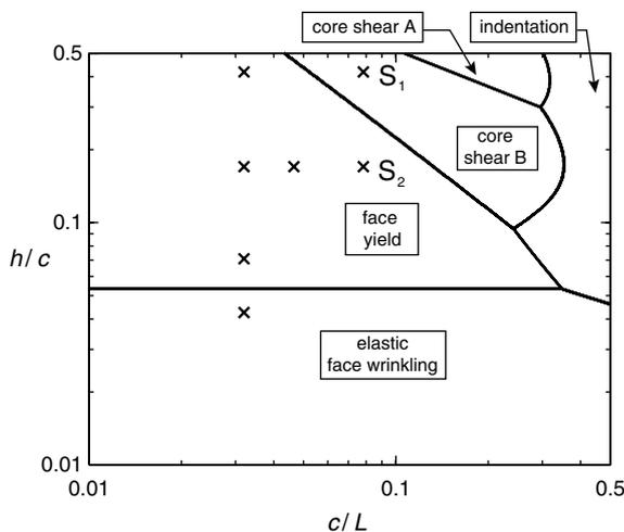
Fig. 11. Failure mechanisms map with  $h/c$  and  $c/L$  as axes for a sandwich beam with AL6XN pyramidal core of relative density  $\bar{\rho} = 0.066$ , using the measured material properties and beam geometries  $H/L = 1/4$  and  $a/L = 1/16$ . The data points denote the tested geometries in monotonic loading. The specimens  $S_1$  and  $S_2$  are also explored in fatigue.
