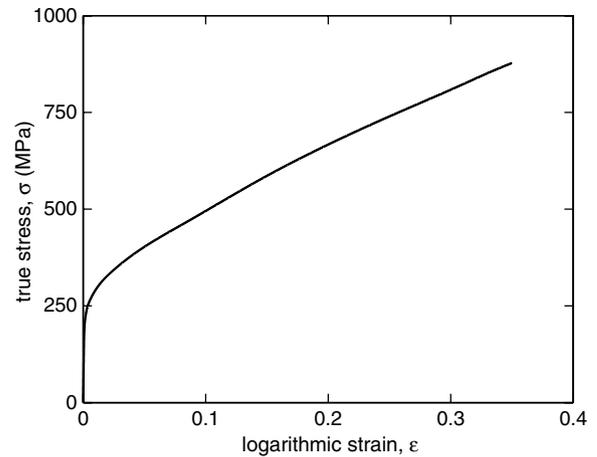
Fig. 8. The measured true tensile stress  $\sigma$  versus logarithmic strain  $\epsilon$  response of 304 stainless steel in its brazed conditions. Measured Young's modulus  $E = 210 \text{ GPa}$  and 0.1% offset yield strength of faces  $\sigma_y = 210 \text{ MPa}$ .
