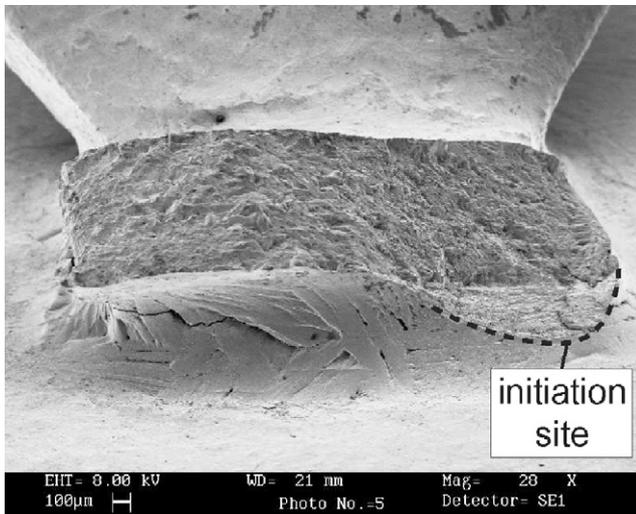
Fig. 17. SEM photograph of fracture surface clearly showing fatigue crack initiation at the toe of the brazed joint.
