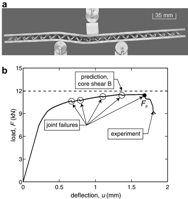
Fig. 14. (a) Photograph of a monotonically loaded deformed specimen  $S_1$  with  $h = 2.95$  mm and  $L = 90$  mm. It collapses by core shear B. (b) The  $F$  versus  $u$  response for this specimen along with the analytical prediction of the collapse strength.
