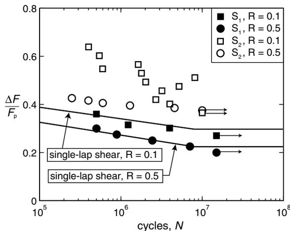
Fig. 18. Fatigue  $S$ – $N$  curves of load range  $\Delta F$  normalised by the peak load  $F_p$  for sandwich beams  $S_1$  and  $S_2$ . Data for load ratios  $R = 0.1$  and  $0.5$  are included. Single-lap shear  $S$ – $N$  curves for the pyramidal core have been transcribed from Fig. 7 for comparison purposes.
