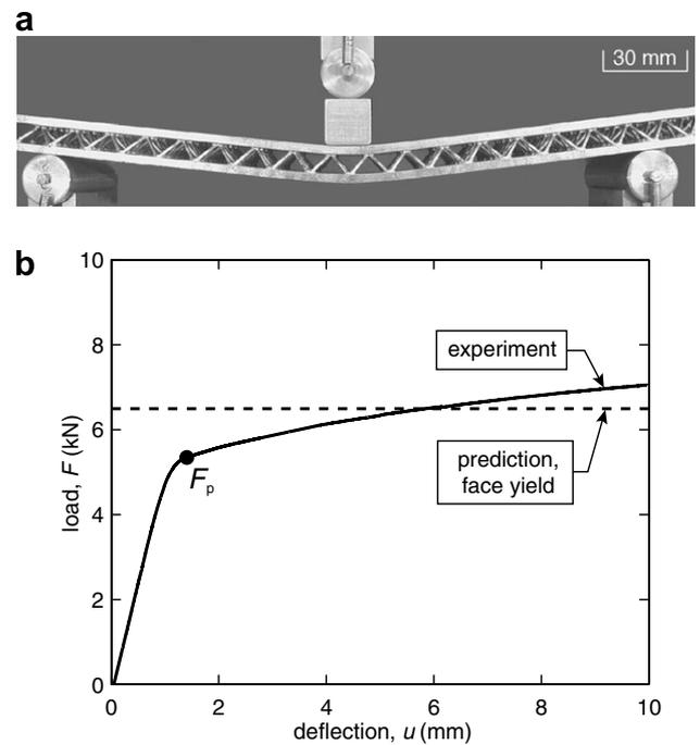
Fig. 13. (a) Photograph of a monotonically loaded deformed specimen with  $h = 2.95$  mm and  $L = 220$  mm. It collapses by face yielding. (b) The  $F$  versus  $u$  response for this specimen along with the analytical prediction of the collapse strength.
