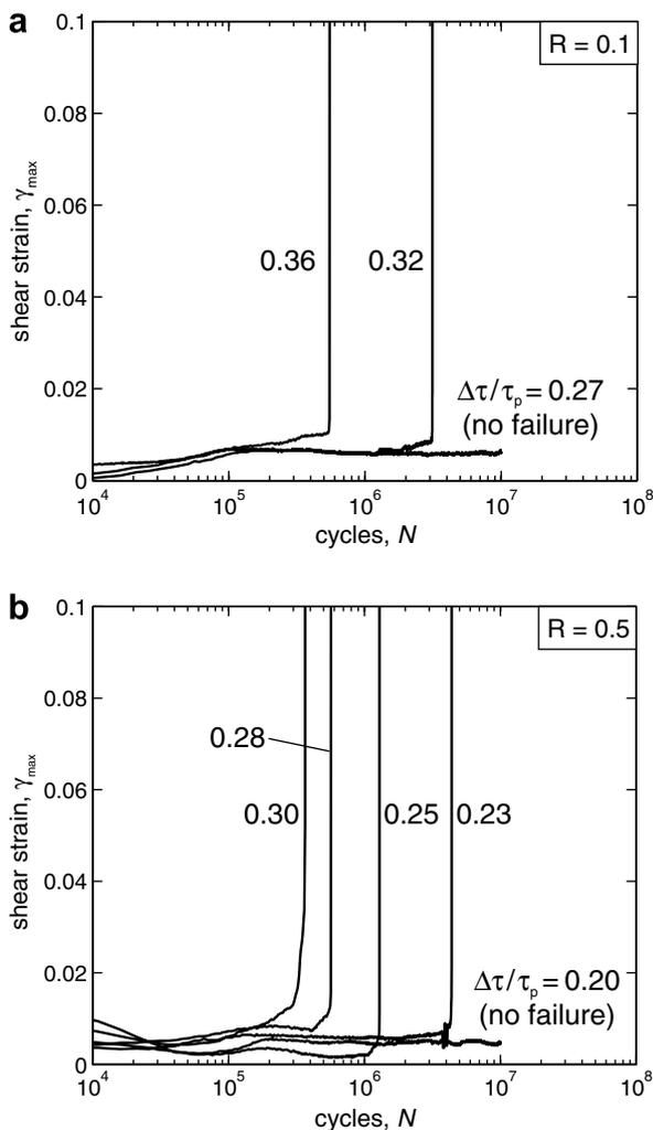
Fig. 5. The accumulated maximum shear strain  $\gamma_{max}$  versus number of cycles  $N$  at selected stress ranges  $\Delta\tau/\tau_p$  and at load ratios (a)  $R = 0.1$  and (b)  $R = 0.5$ .
