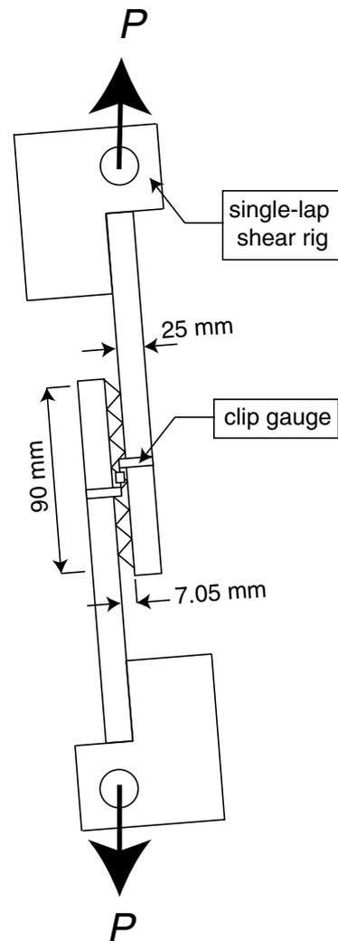
Fig. 4. Sketch of the single-lap shear test rig used for monotonic and cyclic tests.
