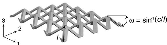
Fig. 1. Isometric view of a rectangular base pyramidal truss core with rectangular cross-section struts.
