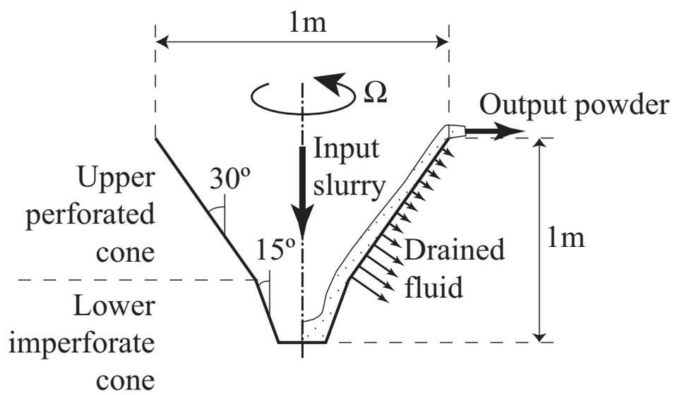
Figure 1: Section of a typical continuous centrifugal filter
