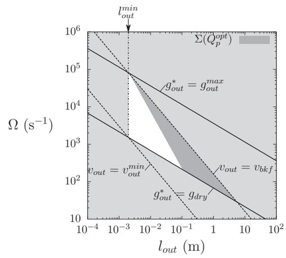
Figure 7: Sucrose massecuite: Envelope design domain, independent of  $Q_p$
