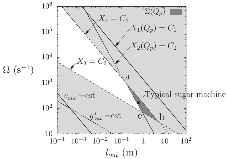
Figure 5: Range of possible basket sizes and spinning velocities for sucrose massecuite with an input powder volumetric flow rate  $Q_p = 2.9 \times 10^{-3} \text{m}^3/\text{s}$
