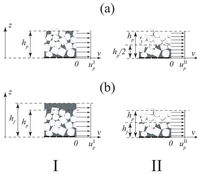
Figure 8: Microstructure considered in regions I and II for (a) equilibrium and (b) fluid conservation
