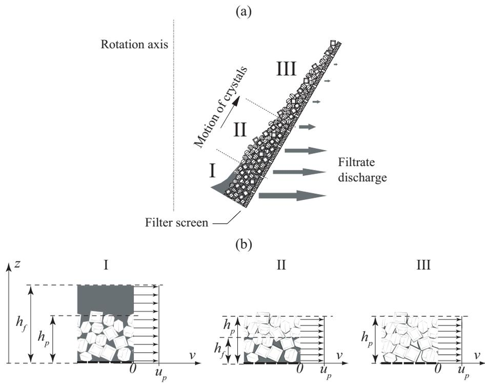
Figure 2: (a) Flow in a rotating perforated cone and (b) microstructure and velocity profile of the solid/liquid/air phases in regions I, II and III for the simple situation where all powder has sedimented before inlet
