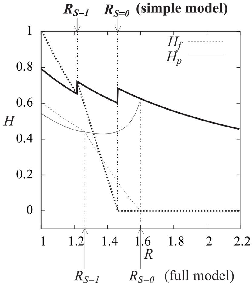
Figure 11: Comparison between the thickness profiles predicted by the complete flow model (thin lines) and the simplified model (thick lines) for typical values of a sucrose centrifuge
