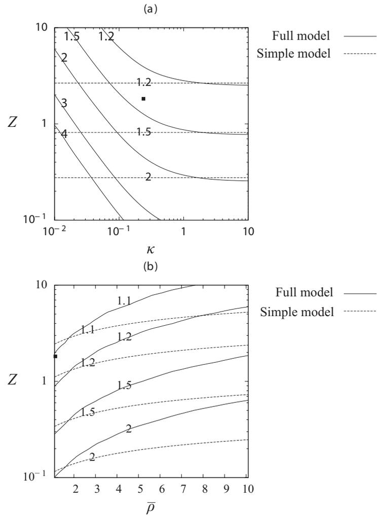
Figure 12: Comparison between the position of the desaturation point predicted by the complete flow model (solid lines) and the simplified model (dashed lines) for typical values of a sucrose centrifuge. The working point of the typical sucrose centrifuge considered earlier is marked with a black square
