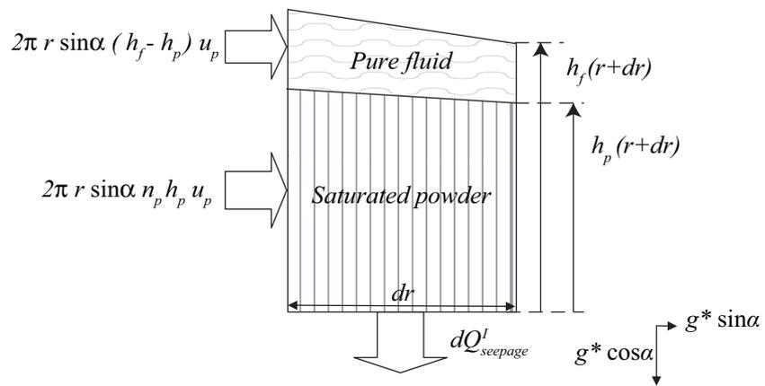
Figure 9: Region I: Volume fluxes of fluid through a control volume of width  $2\pi r \sin \alpha$  and length  $dr$  subjected to a local gravity of amplitude  $g^* = r\Omega^2 \sin \alpha$
