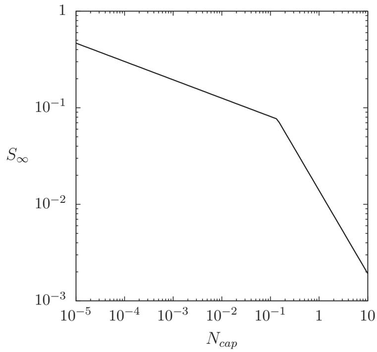
Figure 4: Residual saturation against capillary number (from Wakeman (1977))
