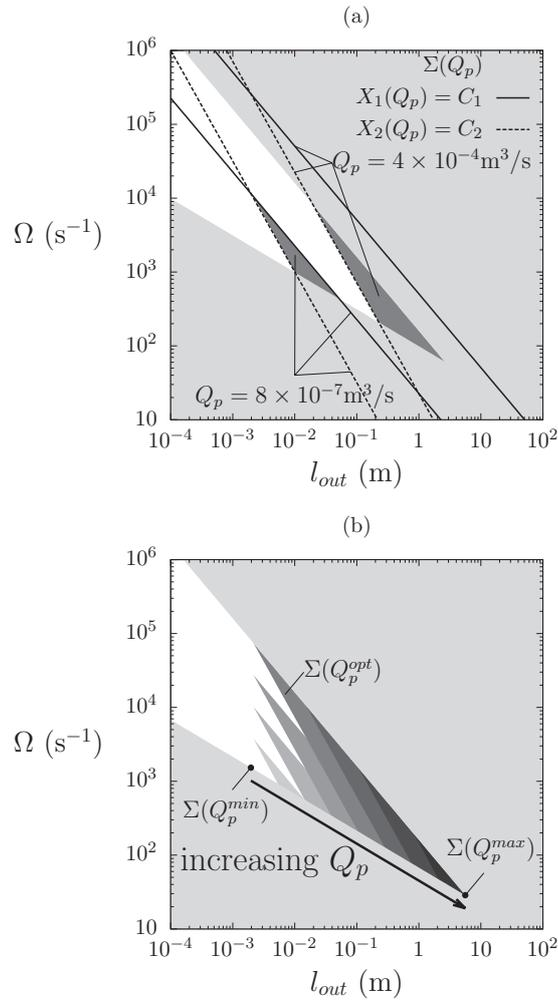
Figure 6: Sucrose massescuite: (a) Construction of the design zone  $\Sigma$  for two different values of  $Q_p$  (b) Evolution of  $\Sigma$  as  $Q_p$  increases
