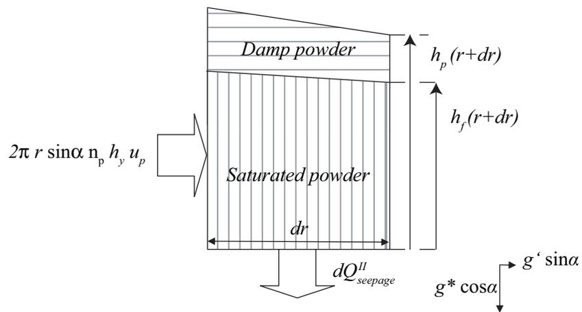
Figure 10: Region II: Volume fluxes of fluid through a control volume of width  $2\pi r \sin \alpha$  and length  $dr$  subjected to a local gravity of amplitude  $g^* = r\Omega^2 \sin \alpha$
