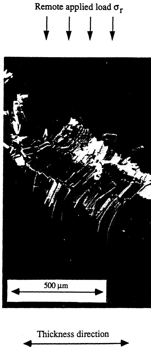
Fig. 14. Multiple kink band formation in an out-of-plane microbuckle. Loading and fibres run in the vertical direction.
